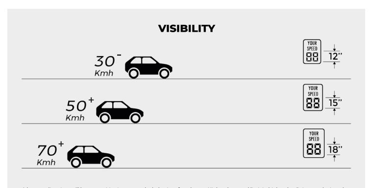
A long reading time will have a positive impact on the behavior of road users. Higher the speed limit is, higher the digits must be in order to give drivers the time necessary to read messages and adjust their speed.
