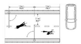
To avoid cyclists bypassing the chicanes, it is advised to install units near a fence or any kind of barrier by a maximum of 0,5 m. If the fence is too far away from the bike path or is simply non-existant, double units (with 2 arms) are to be used instead. They will fill the gap and prevent any possible bypassing.
