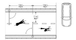
To avoid cyclists bypassing the chicanes, it is advised to install units near a fence or any kind of barrier by a maximum of 0,5 m. If the fence is too far away from the bike path or is simply non-existant, double units (with 2 arms) are to be used instead. They will fill the gap and prevent any possible bypassing.
